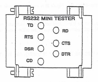
The RS232 mini-tester is highly recommended in assuring the proper installation of the ProtoTRAK LX2 CAD/CAM interface. There are several manufacturers of the testers and they are readily available at local computer retailers. Most versions have seven bi-colored LED lamps that allow you to check the states of the RS232 communications. A representative version is configured as shown above.
